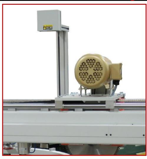
Edgetech's Dual Lasers provides two crisp parallel lines that are spaced the same width as the saw blade. This eliminates any question regarding where the cut will be made, as is the case with laser lines that are wider than the width of the blade. The spacing can be adjusted to match the width of any typical saw blade.
