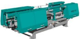
Edgetech's automated postformers are designed for higher volume postforming production. These postformers are continuous, two-sided machines which can form a variety of profiles for many different applications. Specially designed forming roller sections allow the machine to be quickly and easily changed from one profile to another.
