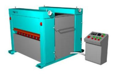
Edgetech's Laminate Pressure Roller/Heat Tunnel is designed to efficiently bond high pressure laminates to panels using modified PVA adhesives. Panels with the laminate applied are fed into a powered set of pressure rollers before passing though the heat tunnel and through a second set of powered pressure rollers.
