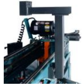
Laser arm mounted on an Edgetech saw
